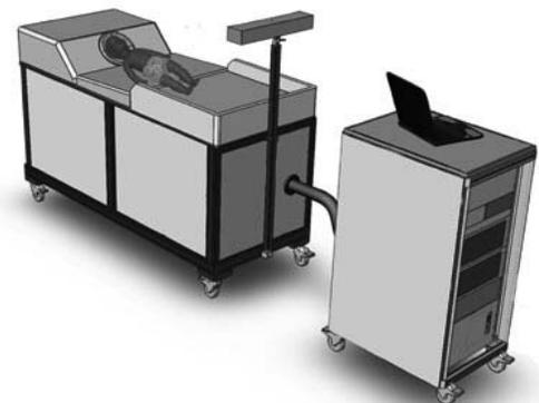
Fig. 6 BabySQUIDprototype, a pediatric MEG system optimized for babies. The 76 MEG sensors are 6 mm below the head rest. (Adapted from Okada et al. 2006).
