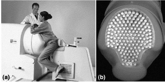
Fig. 2 Fetal MEG system (SARA) manufactured by the Canadian Thin Film, inc. (a) Pregnant mother sits against the sensor array (b) shaped to fit over the abdomen. Sound or light is delivered to the fetus by having a speaker or light emitter applied to the abdomen.
